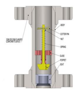
To become a leading entity in this field of Process Industries, **ASVIN** have been engaged in manufacturing **ASVIN Excess Flow Check Valves**, which find their usefulness in food processing, beverage, oil refinery and chemical industries. They are in-line valves through which pressurized gas or liquid flow in either direction. Offered valves are ideal to close upon excessive discharge of liquid or vapor resulting from a break in piping system. Provided
